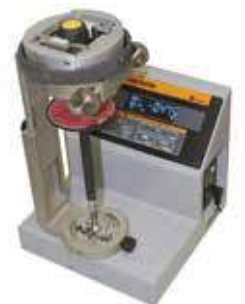
Indicating type FTD with TDT3-G and optional loading device LTA.
