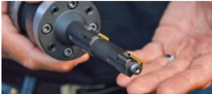
MAPAL custom-designed the combination tool.
