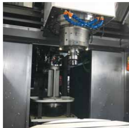
The access of the ATC ARM is done behind the working area
