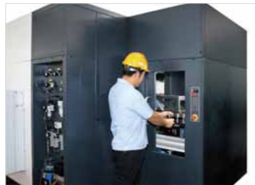
The tool management is then done at the back of the machine.
