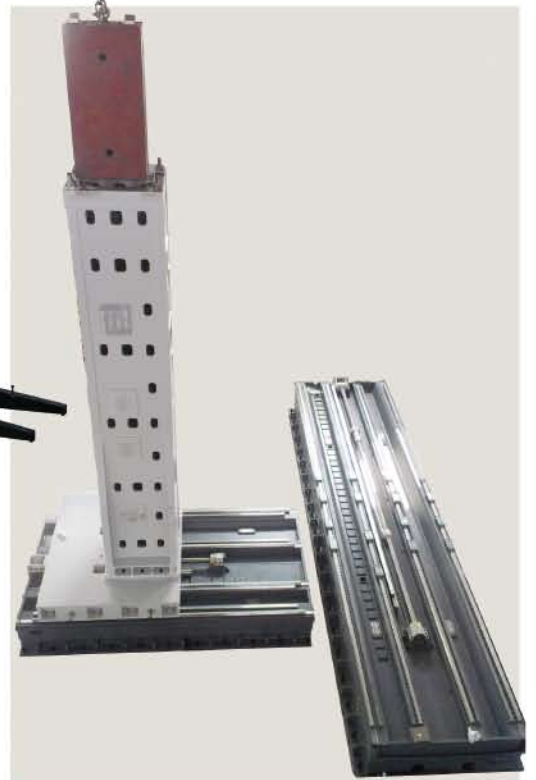
Four-roller type linear guideways for X & Z Axes
