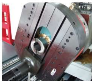
NC contour facing head w/ W axis through
