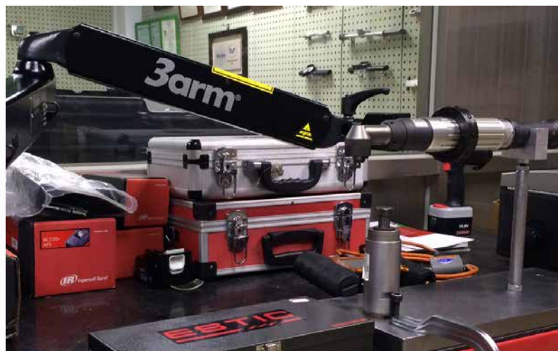
A compact multi-purpose arm for use when brakes are not required
