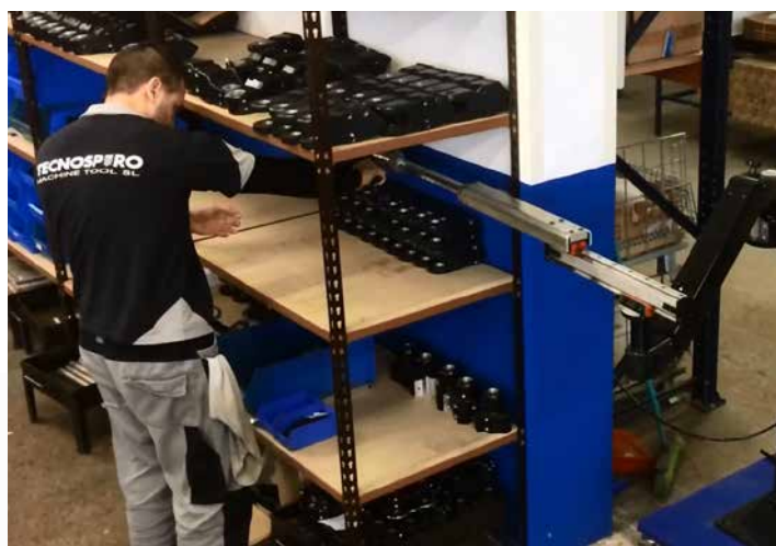
Extended horizontal reach spans more than 2M.
