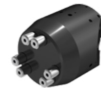
Axial Multi-Spindle Head (6 spindles) Whistle Notch 6 95 mm pitch circle, IC, i = 1:2 for drilling through-holes (5.5 mm)
