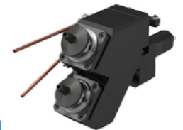
Angled Multi-Spindle Head (2 spindles) BENZ Solidfix® S3 Axle spacing 75 mm, 40°, EC, i = 1:1 1st spindle for drilling pilot holes; 2nd spindle for deep- hole drilling
