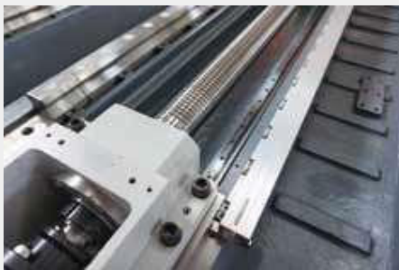
Linear scales are fitted on X, W and Y axes for absolute positioning accuracy.
