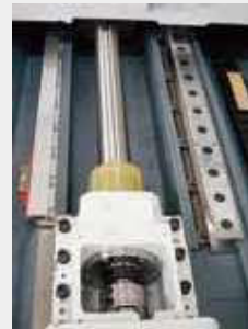
High precision C3 class ballscrews with double nuts are applied on all axes.
