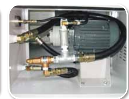
CTS system with high pressure 20bar pump
