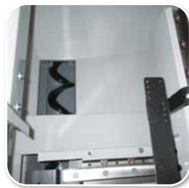
Drainage outlet & Chip auger
