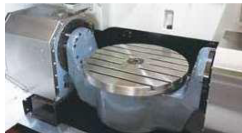
Hydraulic and pneumatic power supplied from table center.
